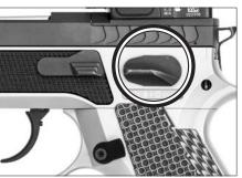
In the «FIRE»-Position the lever is facing forward (horizontally).
