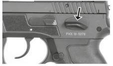
• Slowly pull the trigger. The cocked hammer is released and the cartridge in the cartridge chamber is ignited by the firing pin.
