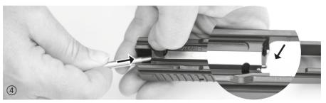
• Afterwards the firing pin and the firing pin safety must smoothly move back into their initial positions. If the firing pin protrusion is too small or the firing pin is sluggish, the firing pin and the firing pin hole in the slide must be cleaned.
